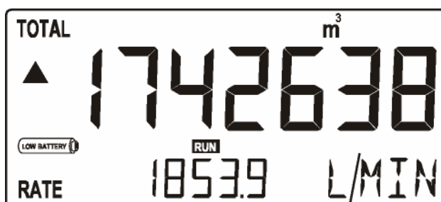
Fig. 4: Example of low-battery alarm.
