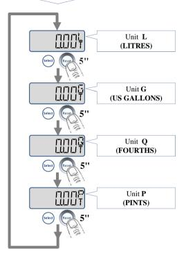
**NB:** the quantity of liquid supplied is automatically converted into different unit of measurement.
