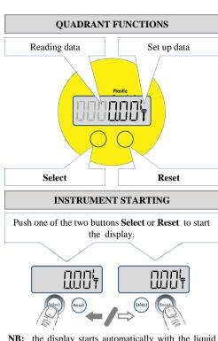
**NB:** the display starts automatically with the liquid flow and stops automatically after about 25 seconds of inactivity.
