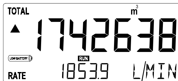
Fig. 4: Example of low-battery alarm.
